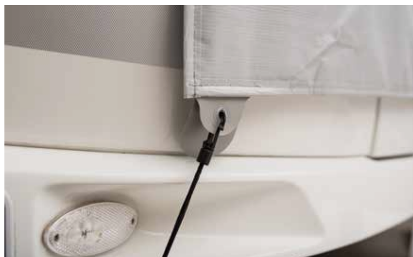
↑ Lashing strap with anti-friction surface
