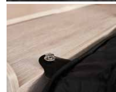
↑ Attached with LOXX press studs to vehicle wall
