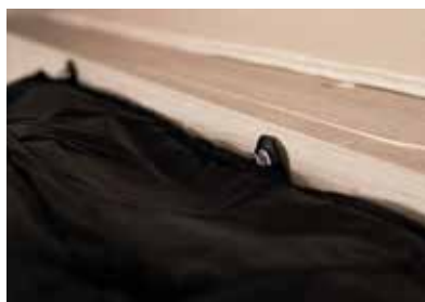
↑ Attached with LOXX press studs to vehicle wall
