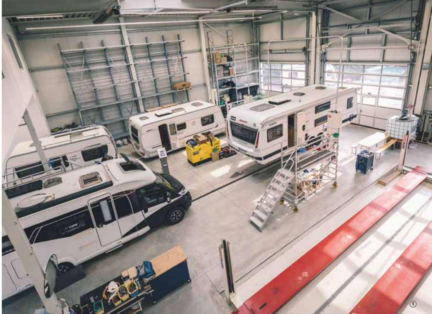
① New workshop section with three lifting platforms, brake tester and training room
