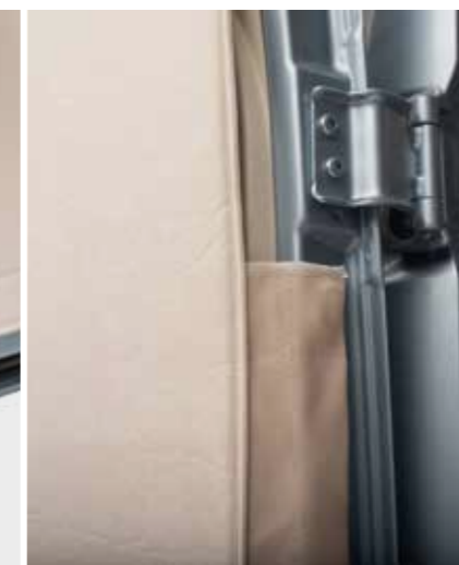
Magnetic fixing door jamb
