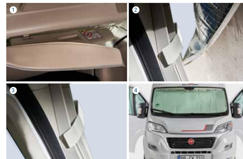
1 Additional stability 3 Meta brackets for magnetic fixing
