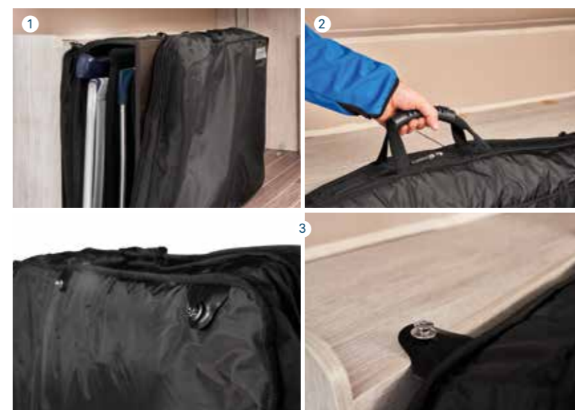
1 Two padded dividers 2 Practical handle 3 LOXX-press studs for attachment to side wall of vehicle
