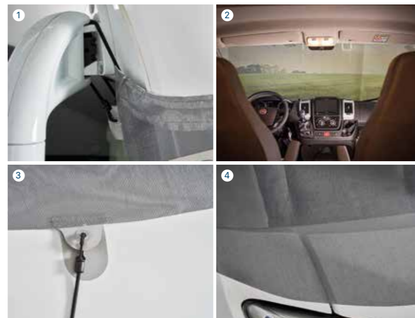
1 Elastic cords for fast attachment 3 Lashing flaps
