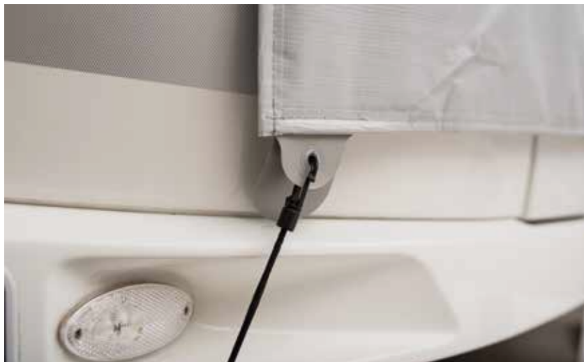
Lashing flaps with paintwork abrasion protection
